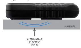
As there is a wide variation in the nominal electrical impedance of different material types, the instrument is provided with five selectable scales with different sensitivities, which are optimized for testing:
